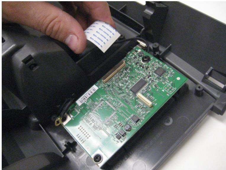
8 Remove the four screws (B) securing the 7" tilting display to the control panel.
