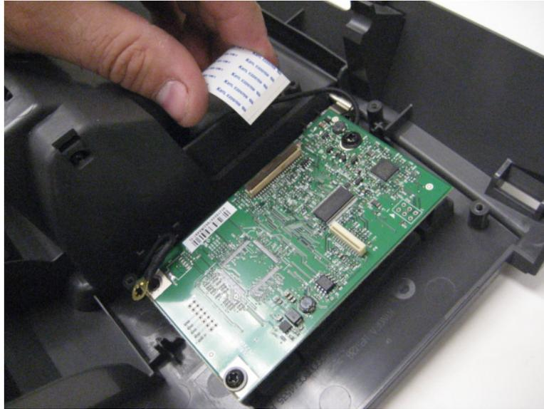
**8** Remove the four screws (B) securing the control panel board (7" tilting display) to the control panel.
