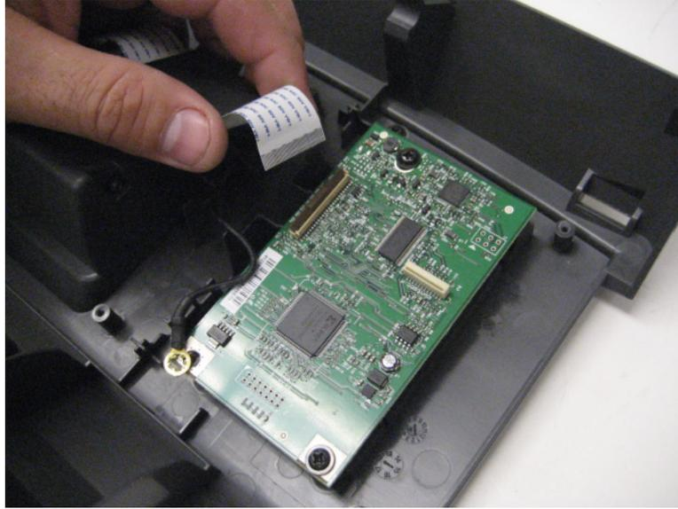
8 Remove the four screws (B) securing the 4.3" tilting display to the control panel.
