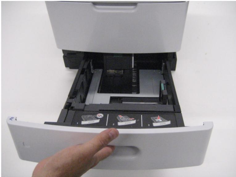
2 Lift the media tray, as shown in the following image, and remove it from the machine.
