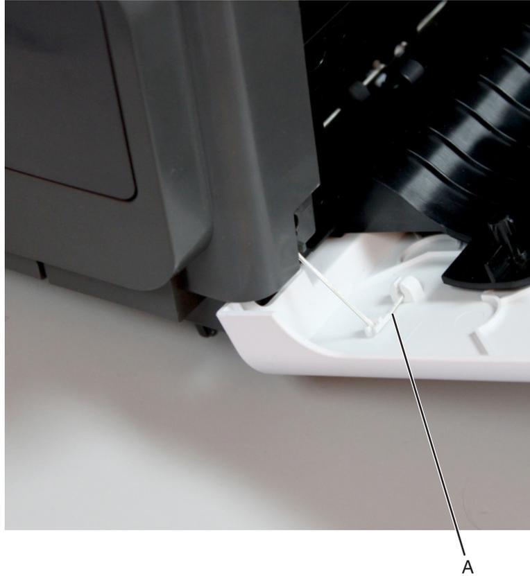
**Installation note:** Fasten the string end (B) to the rear side to prevent it from recoiling into the interior of the finisher.
