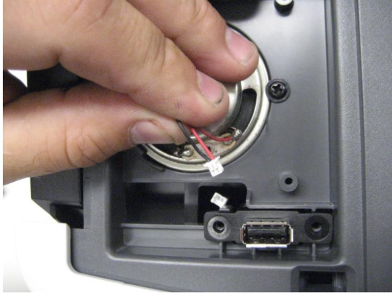
**7** Disconnect the left control panel hinge, and remove the USB cable from the control panel.
