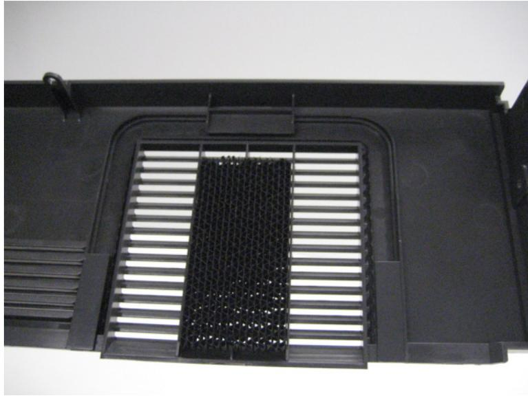
**Installation note:** When replacing the left cover, ensure that the charcoal filter is properly installed.
