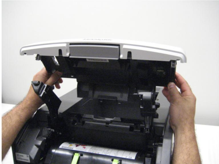
**16** Remove the control panel front cover. See **“Control panel front cover removal”** on page 396.
